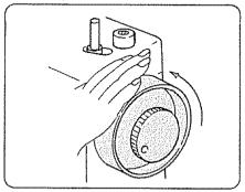
Raise presser foot lever. Hold needle thread loosely in left hand and rotate handwheel toward you one complete turn.
